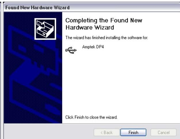
10. Now that the USB driver is installed, browse to the Amptek Installation CD and copy the ADMCA directory to the local computer, to C:\PROGRAM FILES\AMPTEK\ADMCA. Note that ADMCA cannot be run from the CD; it must be installed on a local drive.
