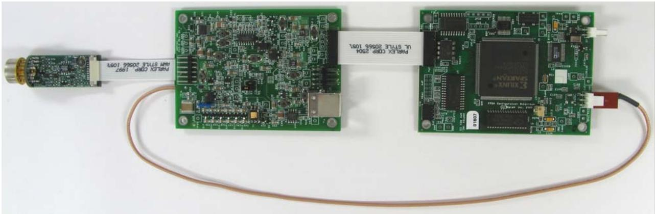
The picture to the right is a close up of the J4A connector, which connects between the PC4-3 and the PA-210, and the OUT connection, which connects with a coax cable to the DP4 input (J7: signal pin 1, shield pin 2).
