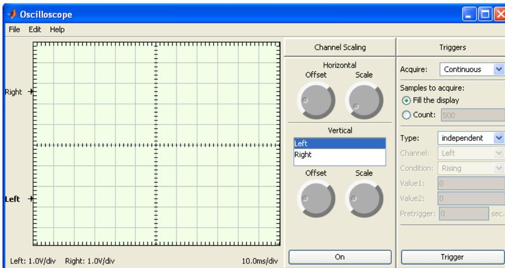
This window provides the Horizontal and vertical adjustment properties under the channel setting and various trigger options.
