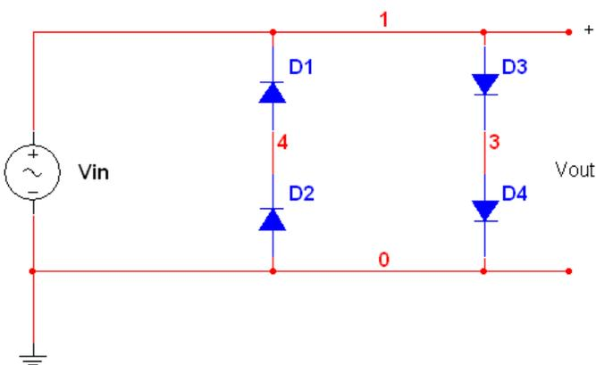
This circuit gives output range between  $+1.4\text{ V} - -1.4\text{ V}$ .
