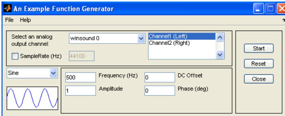
DAQ function generator offers various different waveform production .e.g. sine, square, random, chirp and various other waveforms. User can control frequency, amplitude, dc offset and phase of the output signal (different waveforms have different properties).
