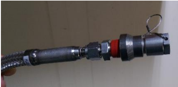
Figure 5. Protecting helium inlet hose with cover
