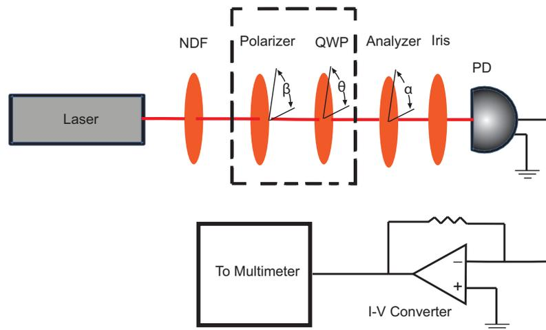
*Figure 1: Setup for the polarimetry experiment. The red line shows the perceived light path. The angles mentioned along with the optical elements are referred with respect to the horizontal axis of the lab. The dashed box shows the section of the apparatus that generates light of some polarization and the Stokes parameters. We use the analyzer to measure this polarization.*
